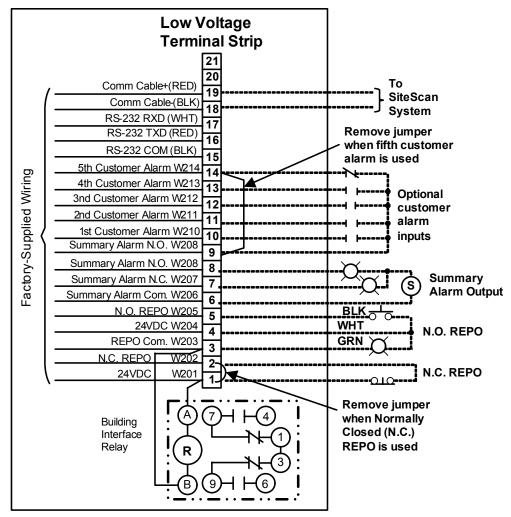
Figure 16 Typical control wiring for units with monitoring
